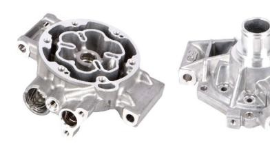
The front cover is usually used for electric magnetic clutch, shaft bearing and rotating shaft, while the back cover is usually for in -out refrigerating medium. We give a step drill to processing the multi-stepped holes at one time. This improves efficiency and reduces the cost of cutting tools.
